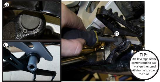
4 One side at a time and starting on the right side, remove the snap ring (a). Push OEM pin inward a bit with extension to get it started(b). Lube the AltRider aluminum hollow pin with grease, and use it to push the OEM pin out the rest of the way.(c). Push AltRider pin completely into place. Repeat for left side.
