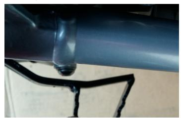
(8) Check brake pedal action for clearance to bolt head. Push pin in further or adjust lever if more clearance is needed.
