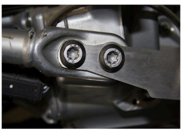
NOTE: If you also purchased AltRider crash bars install them first, reference crash bar instructions and take note that **step #1 is critical.** If you already have AltRider crash bars installed skip to step #3. Place bike on center stand. Remove OEM skid plate and any brackets. Using a T50 Torx driver remove the (2) OEM engine bolts from each side, keep them.
